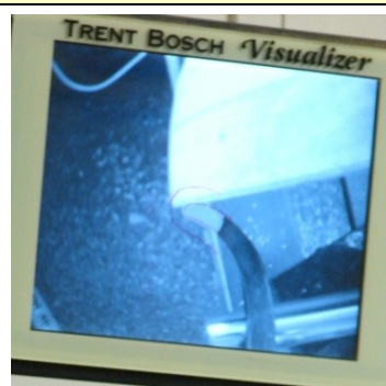
Image of cutter tip about to enter a vessel. Outline around tip indicates desired wall thickness
