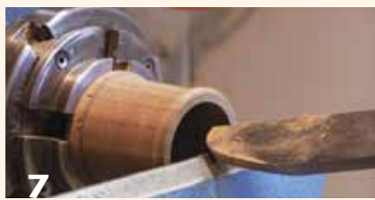
7 Use a round-nose scraper to smooth sides and to create a convex bottom. The sides of the lid should be parallel and roughly \frac{3}{8} " (10 mm) thick.
