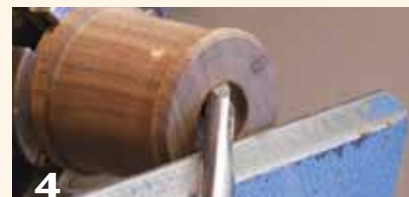
4 Open a hole to approximately 1" (25 mm) in diameter.
