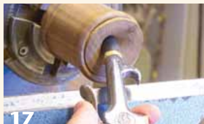
17 Use a rubber-tipped air nozzle—a quick blast will unseat the funnel.
