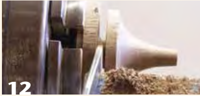
10 Shape the funnel. The tip should be approximately \frac{3}{8} " (10 mm) in diameter.
