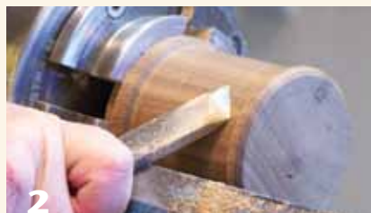
2 Clean up the endgrain and shape a bead at the bottom. Reduce the diameter of the body so that the bead will be raised.
