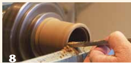
8 Turn a rebate. Use a scraper or a skew chisel.
