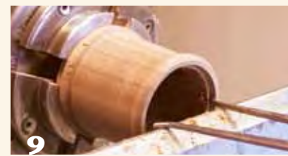
9 Use inside calipers to check that the notch is square sided. This is important, so take your time.
