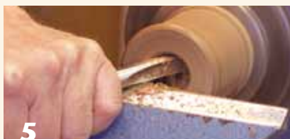
5 Enlarge and deepen the cavity using a back-hollowing cut. Rub the back of the gouge on the smaller opening. The flute should be at about three o'clock, with the top cutting edge engaging the wood between one and two o'clock.
