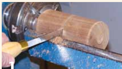
1 After turning to a cylinder, turn spigots on both ends, and part in half.
