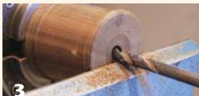
3 Drill a hole that is \frac{3}{8} " (10 mm) in diameter to help establish the inside cavity and make hollowing easier.
