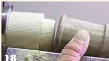
18 Rechuck the body of the shaker. Use either long chuck jaws or a jam-fit chuck. Shape the body, sand, and finish.
