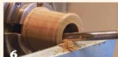
6 Once depth is reached, use gouge to scrape off the 1" (25 mm) opening.
