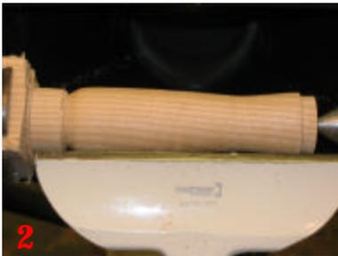
2. Start to shape the handle. The right hand side is left large to fit the metal retainer later. Just shoot for a diameter and shape that feels good, or copy a favorite shape you may already have.
