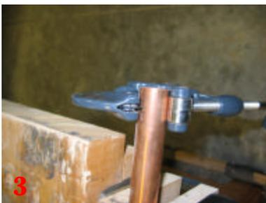
3. Retainer- I used a 12" section of 3/4" diameter copper piping and cut it about 3/4" long off with a tubing cutter (beats a hack saw). Sanded the sharp edges smooth. Other options are threaded nuts, which can be threaded on the handle. Brass nuts can be turned to break off the corners. The retainer just keeps the wood from splitting when the tool is mounted.
