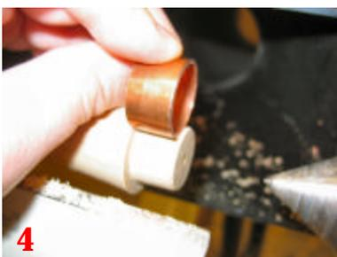
5. Press the retainer on. I used the Jacobs drill chuck to help press it on. I've done some final shaping and started to sand here as well.
