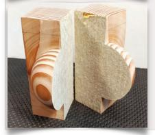
When satisfied with the shape and the flatness of the "wings," I sanded the spherical bowls to 320 grit. I then removed the blank from the lathe, cut off the tenon and used a chisel and mallet to split the blank apart on the glue joint.
