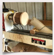
While I do much less sanding on my turnings than I did a few years ago, I still do more than I'd like. I've run a 4" pipe from the lathe to the Jet dust collector which is very effective at eliminating otherwise breathable and harmful sanding dust. A simple bracket made from scrap wood and some large glued magnets and a couple small bungee cords hold the pipe where needed when sanding a piece on the lathe.
