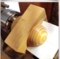
After the glue cured, I mounted the blank in my chuck and tuned the exterior of the bowls. Since the blank was symmetrical, it was balanced and presented no vibration issues.
