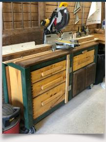
The main woodworking bench frame is made of re-purposed grape arbor 4x4 posts and cedar 2x6's from the arbor. The bench top is 28"x72" and is 3" thick maple and oak. All cabinets, worktables, and power tools are on wheels or casters, and easily moved.
