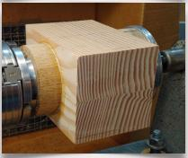
To minimize waste and to have a well balanced configuration, I decided to glue two blanks together using a paper/glue joint that could be parted after the bowl exterior was turned. A bonus of this approach is that one ends up with two, half-completed emerging bowls.
