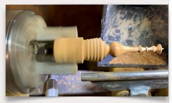
Obviously, I know that there are metal jaws spinning the whole way around, and I have to be careful not to let my gouge or hand(!) come in contact with it. But I am unfamiliar with these jaws, and if I forget, even for a split-second, that the wood near the base isn't as accessible as it looks, I could really make a mess.
