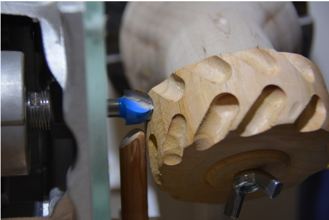
Bit in a tread groove controlled by the guide pin.
