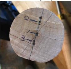
2. Bottom of the figure: to turn the bottom portion from the waist, or hips, to the feet, use the exact center of the piece for the point of the cone center. Mark the length of this part of the figure with a pencil. Cut a tapered shape from the waist to the ankles, then flare out wider for the feet; this part of the figure will be symmetrical. Then shift the cone center 3/8" off center to change the torso shape; this will make the thinner
