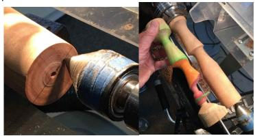
4. Head and Neck: Loosen the chuck and shift the cone center 1/2" to the opposite side of the center hole. Retighten. Check the wood being removed. If not enough or too much, make a minor change in the location of the cone center. This will be cone center point #3. Cut in to form the neck to the desired diameter. Then cut the head to the desired diameter. Keep in mind the proper proportions of the human body for the
