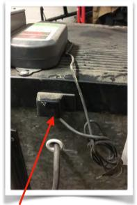
Run the thermostat's sensor wire from the back, underneath the plastic top and down into the interior.
