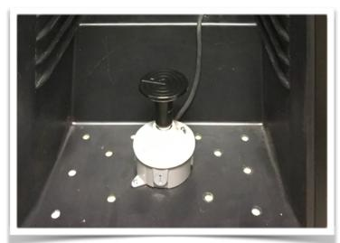
Ceramic Infrared Lamp Bulb - all heat, no light!
