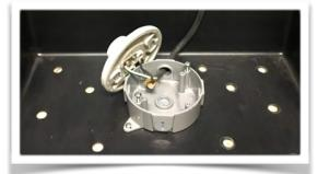
Run the powercord through one of the four holes into the outlet box, attach wires to lampholder, then screw closed.
